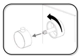
In the event that you should need to remove the flow control valve, first turn off water supply.
