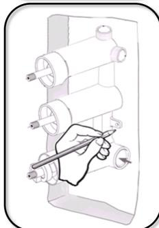
Offer the mixer into the recess and mark fixing locations.
