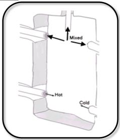
Prepare pipes in wall to connect to shower, with cold on the right.
