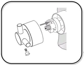
Fit temperature control handle to thermostat, ensuring the stop pin inside the handle, is located against the top of the stop ring.
