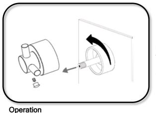
In the event that you should need to remove the flow control valve, first turn off water supply.
