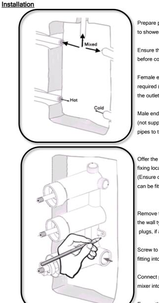
Prepare pipes in wall to connect to shower, with cold on the right.
