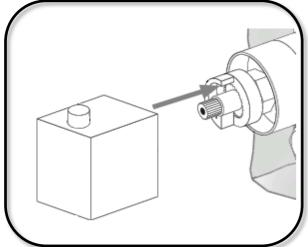
Fit temperature control handle to thermostat, ensuring the stop pin inside the handle, is located against the top of the stop ring.
