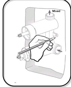
Offer the mixer into the recess and mark fixing locations.
