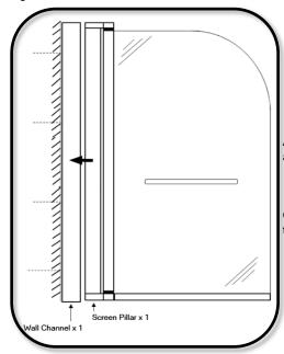
Push the side pillar into the fixed wall channel.
