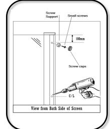
Drill through the wall channel and side pillar from inside the shower screen.
