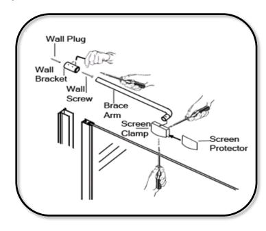
Screw the clamp to the brace arm, place the clamp underneath the end of the arm and insert the screw through the inside of the clamp and into the arm.
