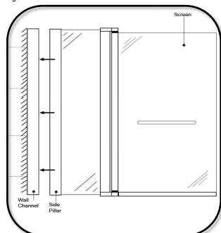
Push the side pillar into the fixed wall channel.
