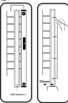
Place the wall channel onto the edge of the bath approx 15mm in from outer edge, against the finished wall surface.
