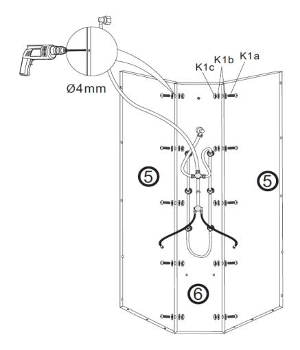
Offer the slide rail (F4) to the centre panel holes and secure the bottom bracket/outlet to the panel using the washer and nut provided.
