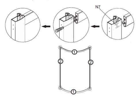
Place the front glass panels (3) into the side profiles, ensuring these are fully inserted push in the glass gasket (L3) between the profile and the glass and push in fully to secure the glass, cut down to suit.
