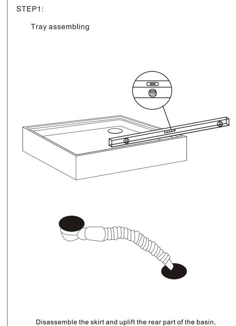
hen insert one end of the pipe into the drainage hole.
