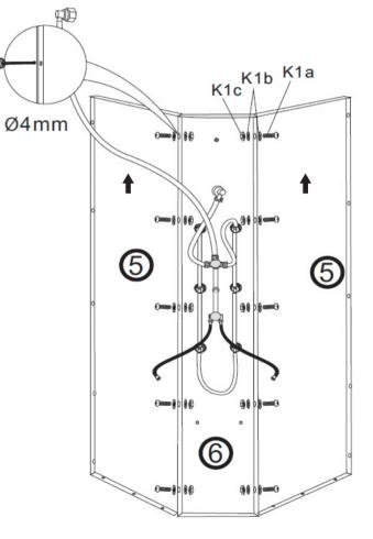
Offer the slide rail (F4) to the centre panel holes and secure the bottom bracket/outlet to the panel using the washer and nut provided.
