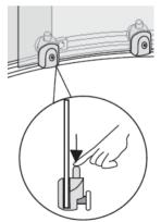
Once the doors are installed, the door stops (J2) need to be fitted. Secure these to the frame using the screws provided (N5) Fit the magnetic door seals (L1) to the edge of the door. The door seals (L2B) should be fitted to the doors, as shown below with the fin facing outward from the tray. Installation - Step 11
