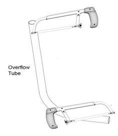
Sealant should be applied between the waste flange and the bath.
