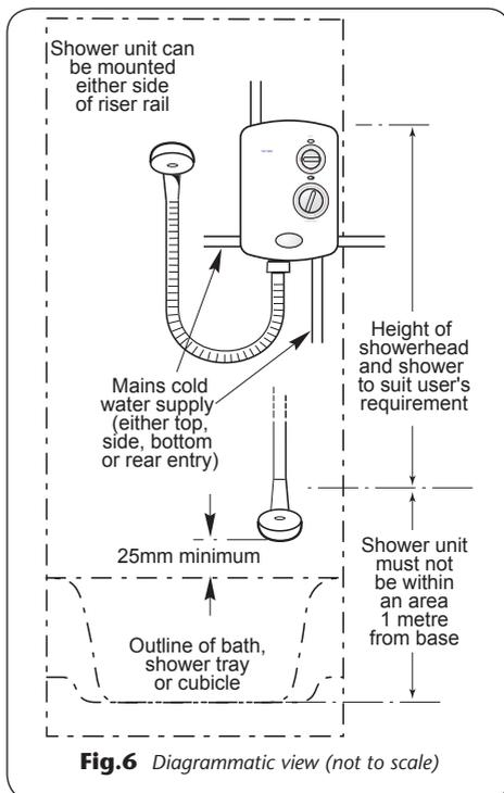
**IMPORTANT:** The unit must be mounted on a flat surface which covers the full width and length of the backplate. It is important that the wall surface is flat otherwise difficulty may be encountered when fitting the cover and subsequent operation of the unit may be impaired.
