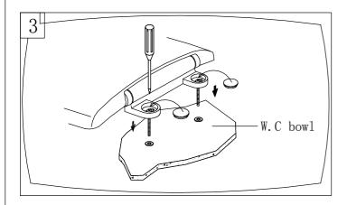
3. Place the seat cover to the pan and line up the hinge and the holes on the pan. Make the necessary adjustment to the fittings so that the seat sits correctly on the toilet. Once correctly positioned, use screwdriver to fit the screws to the plugs. Then push the hinge cover into the hinge.
