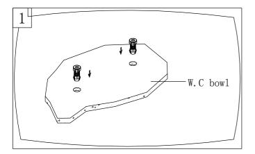
1. Push the plug into the holes on the toilet pan tightly.
