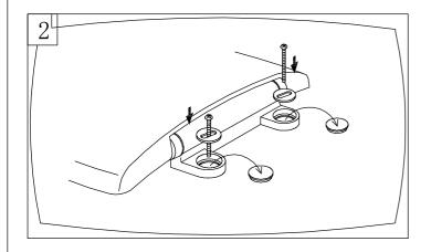
Remove the hinge cover from the seat cover Place the adjustable plate into the seat Place the screw into the adjustable plate
