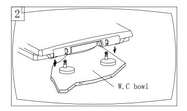
2.After completing step 1 and checking again that the holes on the seat align with the pins on the hinge. Push the seat onto the pins until it clicks into place.
