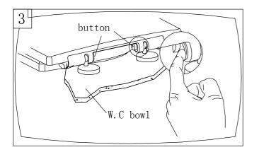
3.To remove the seat, push both buttons on the seat and lift upwards.
