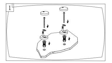
1.Fit the adjustment plate into the hinge,then place the screw through this assembly.Before full tightening, make the necessary adjustments to align the pins with the seat and so that the seat fits correctly on the toilet. Push the plugs through the holes in the toilet and then to tighten the screw into the plug until secure.Then fit the hinge covers.
