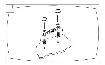
1.Locate adjustment plate and screw into fixing plate. Push the expanding plugs into the holes on the toilet. Locate the screws into the plugs and tighten, before fully tightening make any necessary adjustments to align the seat on the toilet.
