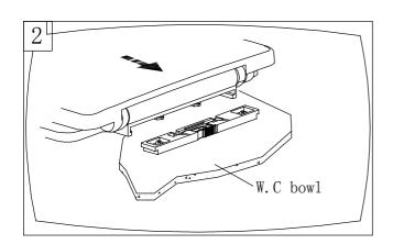
2. Slide the seat on to the fixing plate until fully located.
