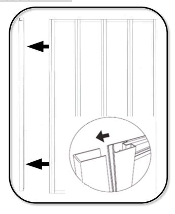
Once the wall channel has been secured, lift the door onto the bath and push the profile into the wall channel.
