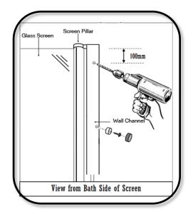
After positioning the door within the wall channel, the assembly needs to be secured together.
