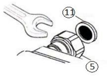
Removal of the mixer from the wall is required, turn off water. Spanner the mixer nuts on the valve to release the mixer from the supply connections.
