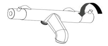
To control the flow of water and to turn on and off, turn the handle on the left, away from the user to increase flow.
