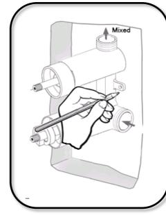
Offer the mixer into the recess and mark fixing locations.
