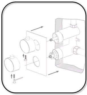
Once the mixer has been fitted and secured, push the concealing plate over the mixer body, sealant should be applied between the plate and the wall.
