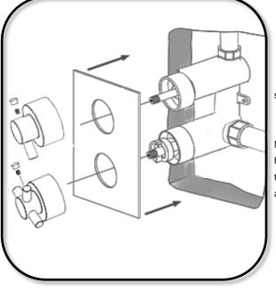
Once the mixer has been fitted and secured, push the concealing plate over the mixer body, sealant should be applied between the plate and the wall.
