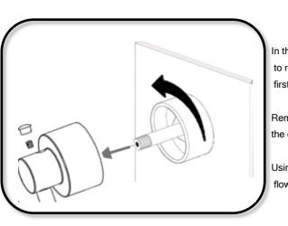
Flow control / diverter valve removal
