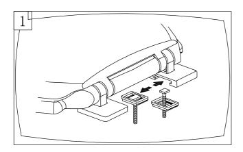
Fit the screw through the adjustment plate
