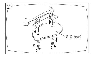
2. Place the assembly onto the toilet and push the screws into the holes, Make the necessary adjustments to the fittings so that that the seat sits correctly on the toilet. Once correctly positioned fit the gasket and nut and secure the seat. Take care not to overtighten the fittings as doing this can crack the fittings
