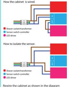
Rewire the cabinet as shown in the diagram above. HiB recommends that all electrical bathroom products should only be fitted by a suitably qualified, Part P registered electrician.
