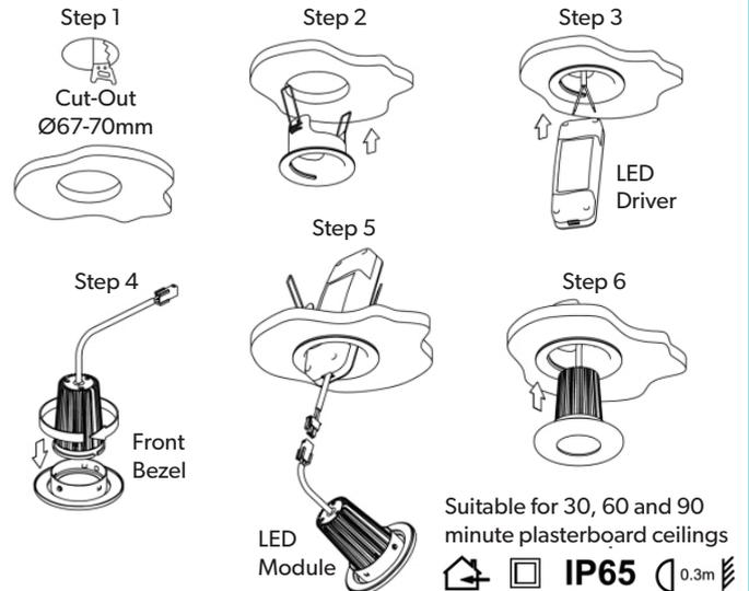
1. Position the LED Showerlight in a suitable location (according to the zonal diagram opposite - Fig. 1), ensuring that the domestic electrical mains supply is within reach of the electrical entry point of the product.
