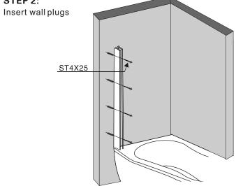
Position wall channel over holes. sealant can be applied between the channel and the wall.
