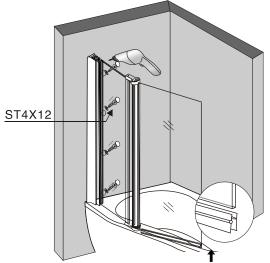
Drilling through from the inside through the wall channel and glass profile a 3.2 mm drill bit.
