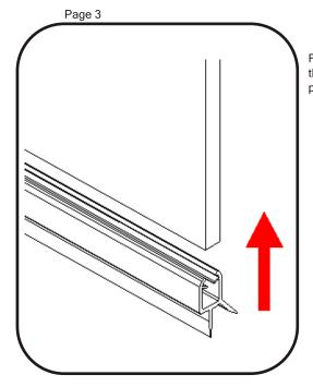
Fit the rubber seal to the bottom of the screen, ensuring it is fully pushed onto the glass.
