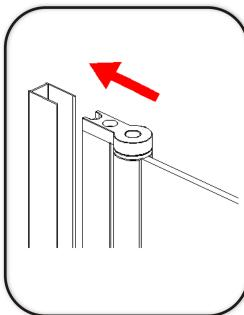
Push the side pillar into the fixed wall channel.
