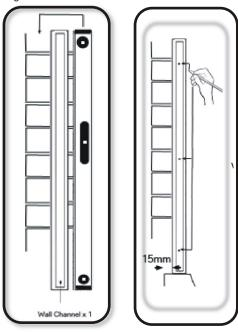
Place the wall channel onto the edge of the bath approx 15mm in from outer edge, against the finished wall surface.
