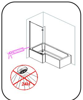
Seal along the side of the wall channel, along the bottom edge of the wall channel and around the pivot joint.
