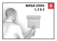
Repeat steps 1, 2 and 3 to repair and strengthen hairline superficial cracks in the body of the wall or floor. Allow to dry for 2 hours. Also repeat similar for boarded backgrounds along the joint between boards.
