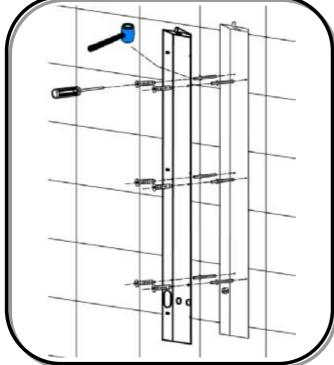
Offer the fixing frame to the wall and secure using the screws provided.
