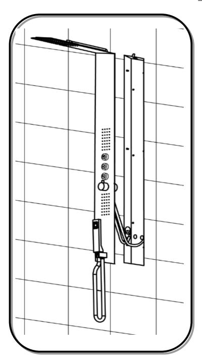
Connect red and blue flexi-tails to hot and cold supply connections.
