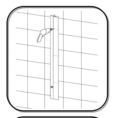
Drill the holes into wall through the holes on the fixing frame.
