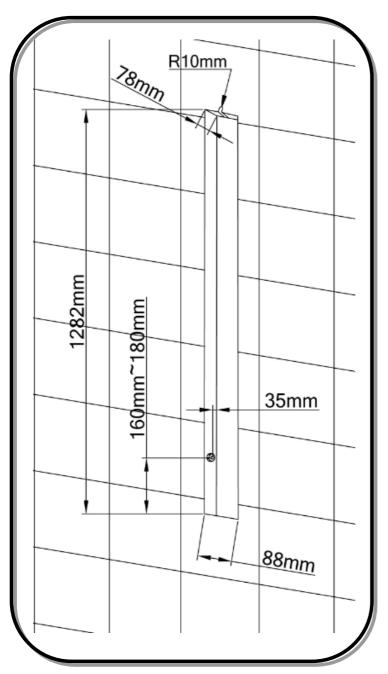
Greate a cavity in the wall to dimensions 1282mm×88mm×78mm to secure the fixing frame.
