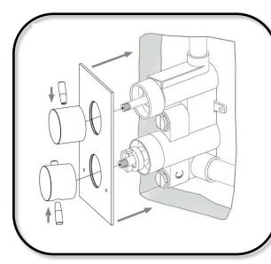
Once the mixer has been fitted and secured, push the concealing plate over the mixer body, sealant should be applied between the plate and the wall.
