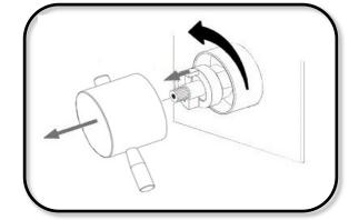
Run this under warm water and rub or wipe to remove build up.
