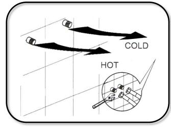
Connect red and blue flexi-tails to hot and cold supply Tighten all connections
