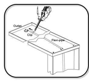
Feed the long flexi-pipe through the larger hole in the centre of the panel.
