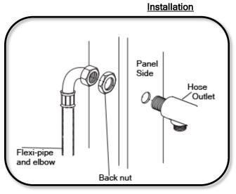
Place outlet thread through side of panel and connect nut. Ensure washer is fitted in elbow and connect to thread
