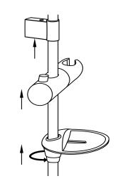
Place the round chrome nut onto the rail. Fit the brass adaptor with o rings into the end of the rail and tighten using an allen key. Fit rubber washer into the chrome nut. Connect diverter to the rail nut and tighten, ensure that the diverter is aligned with the rail.
