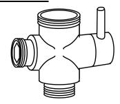
Place seals into hose ends. Connect long hose to thread to side of diverter.
