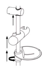
Place the round chrome nut onto the rail. Fit the brass adaptor with o rings into the end of the rail and tighten using an allen key. Fit rubber washer into the chrome nut. Connect diverter to the rail nut and tighten, ensure that the diverter is aligned with the rail.
