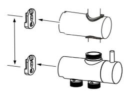
Once positioned correctly secure the top bracket to the rail, by tightening the screw into the back of the bracket, ensure that the black rubber plug is fitted or the screw will damage the rail, do not overtighten
