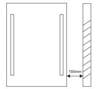
Ensure the sensor are positioned at least 150mm away from any solid surface including walls.
