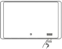
a) Press and hold the left button till the Hr/Min digits flash.
