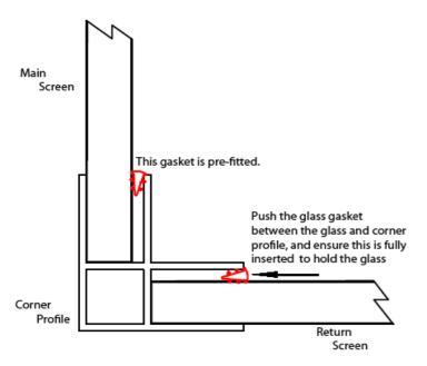
The corner profile will be received fitted to the main screen.
