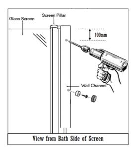
Drill through the wall channel and profile from inside the shower screen.
