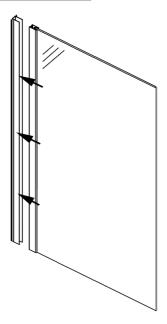
Slide the main screen into the wall channel.
