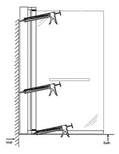
Once the assembly is completed, you should then seal the outside only of the screen.
