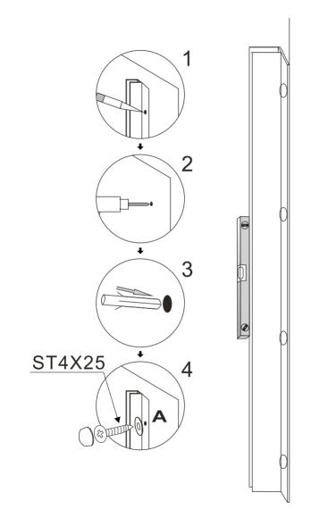
Point 1 and 4: the screws should be fitted to the inside
