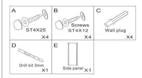
Plugs and drill bit are supplied, these are suitable for masonry and so a suitable bit and plug should be used or your wall type
