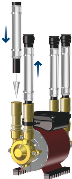
Fig. 17 Fitting the strainer basket
