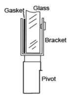
Push the door into the top and bottom hinge and align so that the door closes correctly.
