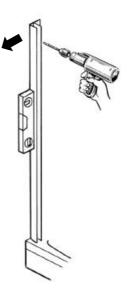
After drilling, insert wall plugs and tap in so flush with finished wall. Hold one wall channel against the wall over the drill holes Screw the wall channel to the wall ensuring to fit washer onto screw M4 x 25, to allow fitting of the screw cover.
