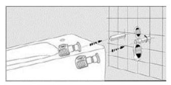
**Please note:** The cut out on the connector and the hole in the housing should be aligned.
