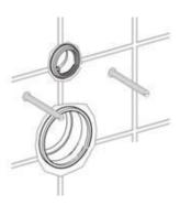
3. It is advisable to apply a small amount of lubricant (washing up liquid) to the flush pipe and pan connector to assist with fitting the toilet pan.
