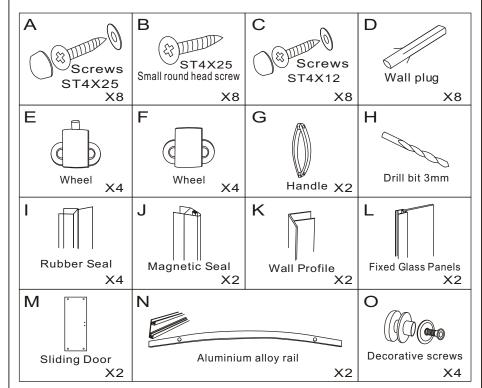
Plugs and drill bit are supplied, these are suitable for masonryand so a suitable bit and plug should be used or your wall type
