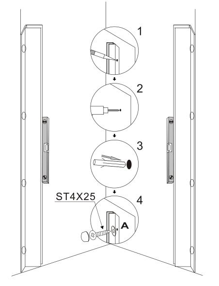
Point 1 and 4: the screws should be fitted to the inside
