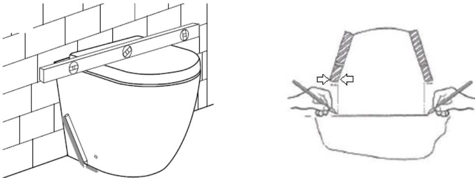
4. Remove the pan from the location, turn over, then measure the thickness of the toilet side wall and make another mark in from the original mark, and in line with the fixing hole, as shown below. Repeat on the other side.
