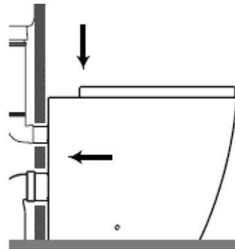
9. Once aligned, secure the toilet pan into position using the fixings provided, do not overtighten. Finish by pushing on the screw covers.
