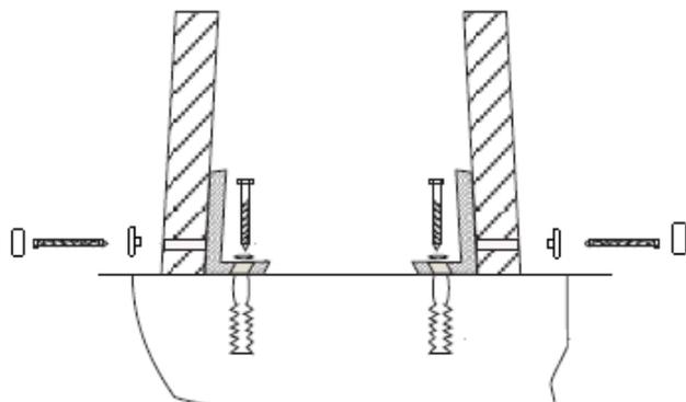
10. Once the installation is completed, a small bead of silicone can be applied around the bottom edge of the toilet pan.
