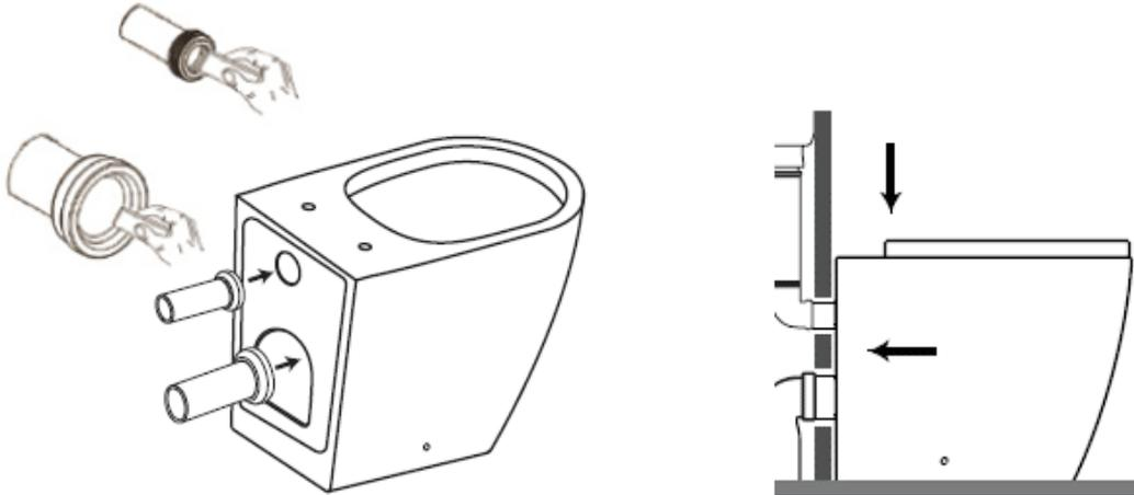
3. Ensure that the toilet pan is level and backed fully against the wall / WC unit, then mark on the outer edge of the pan (at both sides), align with each fixing hole located in the side wall of the toilet pan.
