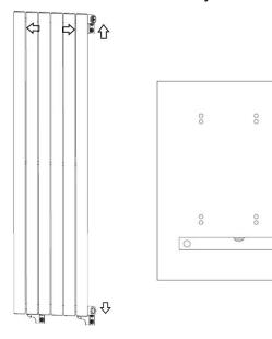
3. Using the drill and 8mm drill bit, drill into the marked positions then insert the wall plugs and tap flush to the finished wall surface.
