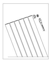
2. Set the position of the wall hanging brackets (on the wall) in relation to the size of your radiator, the brackets should be located between the last bar and the second bar in, as shown. Mark these positions on the wall in the required location and use a spirit level to ensure that these are horizontally and vertically aligned.
