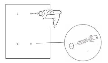
**Please note:** If drilling into a tile, it is recommended to tape the wall to prevent the drill from slipping.
