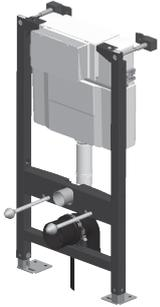
1 a WC Frame with Dual Flush Cistern (incorporating 1 No. Universal Ball Valve 1 No. Wire Activated Siphon, 1 No. Brass Water Inlet Valve & 1 No. Universal Filling Hose)
