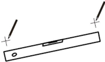
Drill the wall at the marked points on the wall for your required orientation and insert the wall plugs and tap until flush with the finished wall surface.
