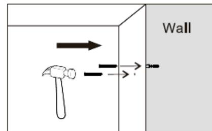
After fitting the wall plugs, insert the screw and tighten, DO NOT tighten the screw fully to the wall surface.
