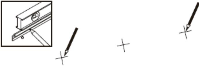
Drill the wall at the marked points on the wall for your required orientation and insert the wall plugs and tap until flush with the finished wall surface.
