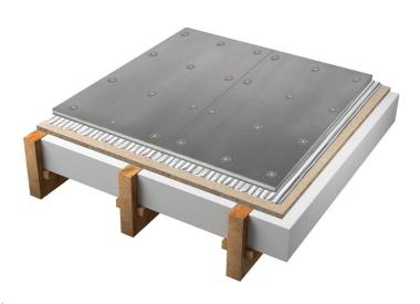
**STEP 4 -** When the adhesive has cured, the boards should be secured using screws and washers. These are installed at the rate of 12 per board (3 rows of 4). The screws should be a minimum of 30 mm from the edge of the insulation board. Tighten the screw and washer into the board until the screw head is flush with the surface.
