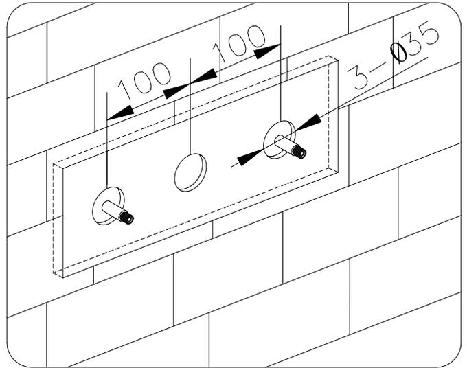
Fix the decorative base onto the spout. Install the spout using thread seal tape.
