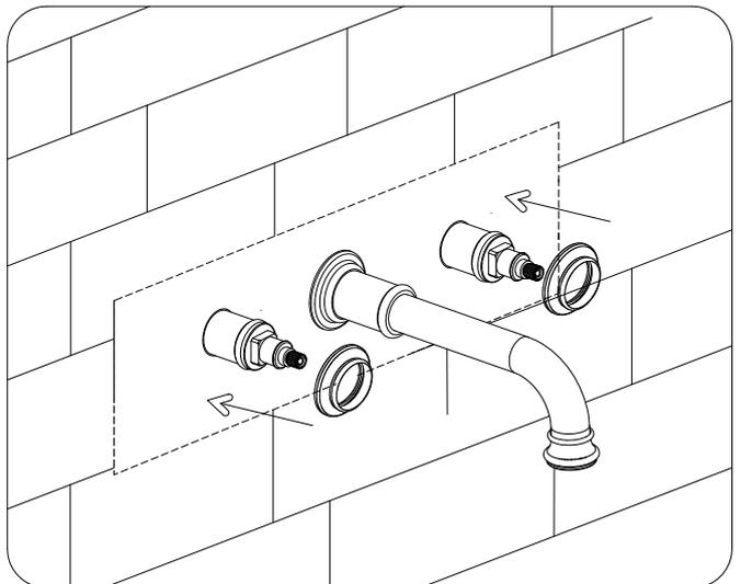
Install the lever handles and adjust to the correct positions. Securing them with the grub screw and then fix the ceramic cap.
