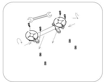
Thrust the connectors(6) vertically into the two inlet holes of the body(11). Press the locknut(5) onto the body. Fix and fasten the screws(4) with allen key.
