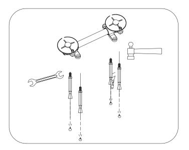
Remove the screws(7) with allen key, take out the cover templates(8).
