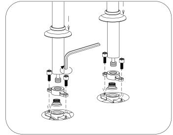
Fix the Standing Pipes(1) with Body (11) Slide down the bases(2)until they reach the floor. Waterproof adhesive is recommended to be applied.
