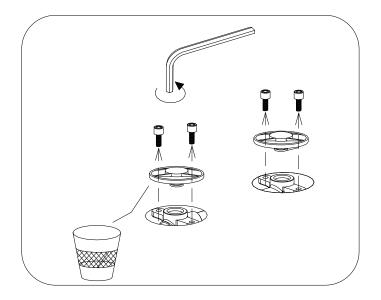
Fix the G3/4 connectors(12) with inlets of the body(11).Thrust the body over floor screws(10) and fasten with steel plate and nut(10). Connect the body(11) with hot (left) and cold (right) water pipes using thread seal tape.
