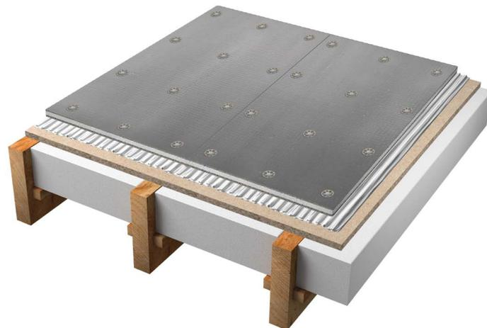
**STEP 4** - When the adhesive has cured, the boards should be secured using screws and washers. These are installed at the rate of 12 per board (3 rows of 4). The screws should be a minimum of 30 mm from the edge of the insulation board. Tighten the screw and washer into the board until the screw head is flush with the surface.
