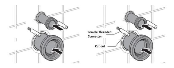
5. Insert the plastic wall mounting housing into the holes in the rear of the toilet pan and align the hole with the fixing hole on the top face of the toilet pan.
