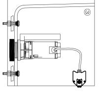
Nest the Tank To Bowl Washer in the Lock Nut and position the TANK on the Toilet Bowl properly. Disassemble the Tank To Bowl Bolts. Fix the Tank to Toilet Bowl with the Tank To Bowl Bolts tightly.
