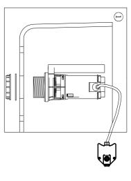
Disassemble Hexagon Nut for Valve installation. Position the VALVE inside the TANK. Push down on the Valve Body while tightening the Hexagon Nut from outside.
