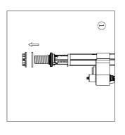
Disassemble the Lock Nut for valve installation.
