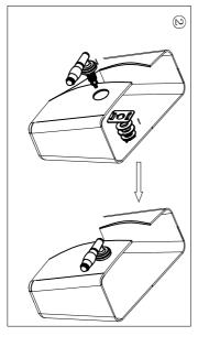
Install the lever in the front hole and fix the nut properly.
