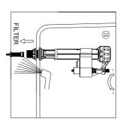
Adjusting water level by screwing Float Bolt and move the Float Housing up or down along the Valve Body to join with the Float. Pay attention the Float Housing should be attached to the Float and the Arm isn't raised. Take out of the Filter and clean it often.
