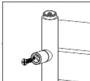
6. Align and push the rail brackets on the radiator onto the wall brackets secured to the wall. Secure the two together with the connecting screws provided (insert through the slot in the bracket) and tighten using the Philips screwdriver, be sure not to overtighten.
