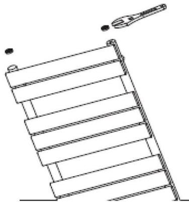
2. The rear of the towel rail has four location holes to fix the brackets. Measure the distance between all the location holes and mark these on the wall in the required location, use a spirit level to ensure these are horizontally and vertically aligned.
