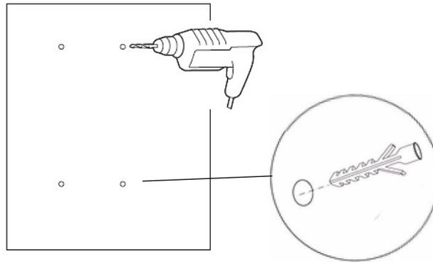
**Please note:** If drilling into a tile, it is recommended to tape the wall to prevent the drill from slipping.
