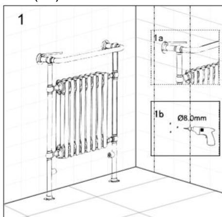
**Please note:** If drilling into tile, it is recommended to tape the wall to prevent the drill from slipping.
